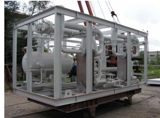
Heat exchanging modules used in power units
